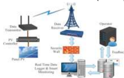
Figure 4. Smart Grid Network Monitoring System Topology
