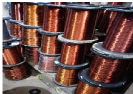
Figure 4. Enamel wire (copper wire coated with insulating material)
