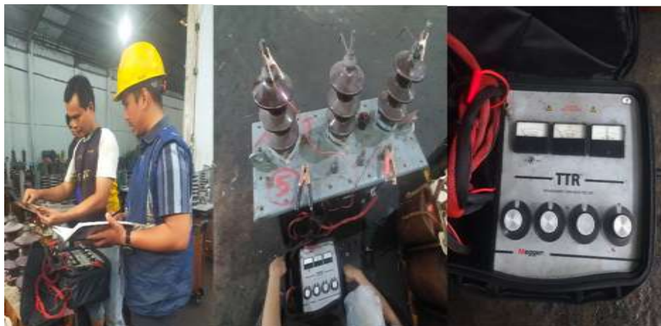
Figure 5. Measurements to find damage to the transformer
