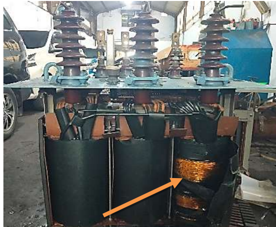
Figure 6. Damaged primary coil of transformer
