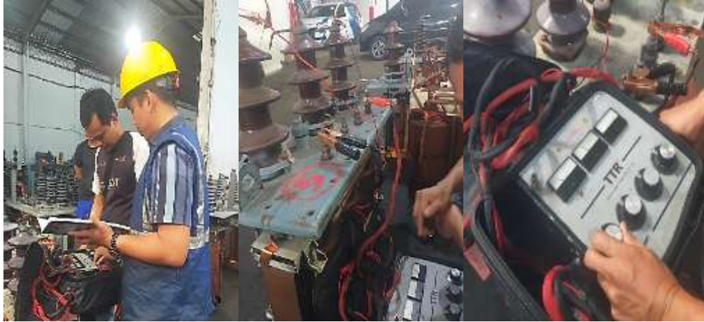
Figure 9. Measurement after replacing the winding coil
