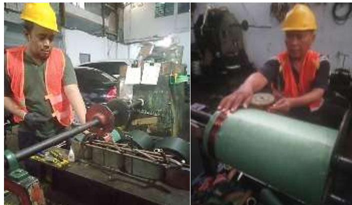
Figure 7. The process of rewinding transformer winding coils
