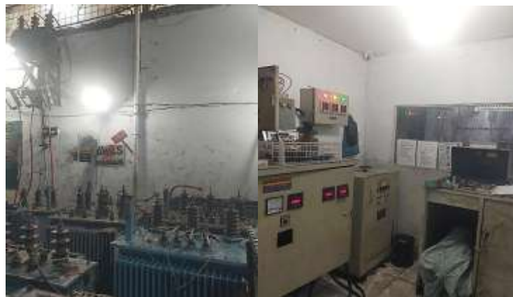
Figure 10. Testing after replacing the coil winding
