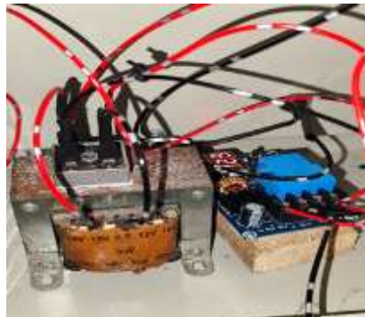
Figure 12. Physical Form of Charger Control Circuit
