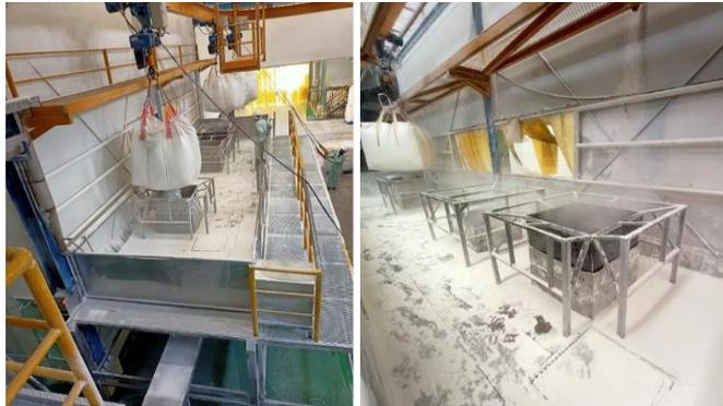
**Picture 5:** Big Bag Pouring Process at the Dumping Point
