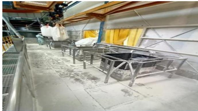
**Picture 2 : Flour Pouring Equipment in Dumping**
